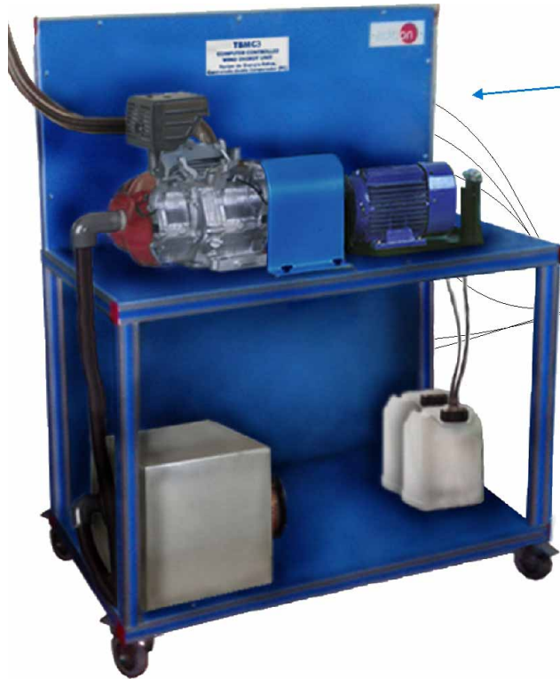
① Unit: TBMC3. Test Bench for Single-Cylinder Engines, 2.2 kW.
