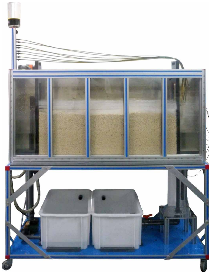
① Unit: PDFDC. Drainage and Seepage Tank
