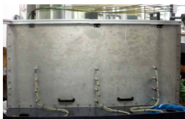
Detail of the back side (pressure sensors)
