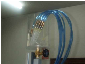
Detail of the dye injection system
