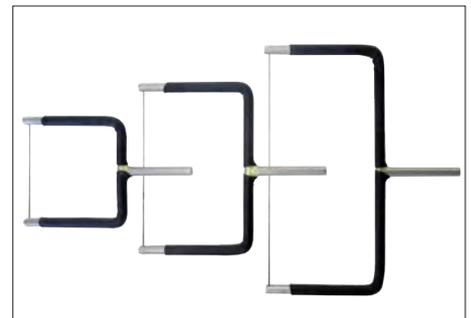
Detail of the exchangeable cathodes with support
