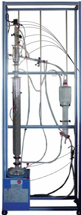
① Unit: UDDC. Batch Distillation Unit
