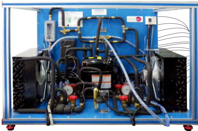
① Unit: THIBAR22C. Heat Pump+Air Conditioning+Refrigeration Unit with Cycle Inversion Valve (two condensers (water and air) and two evaporators (water and air))
