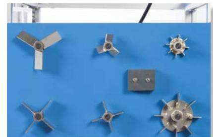
The panel with the different types of agitators
