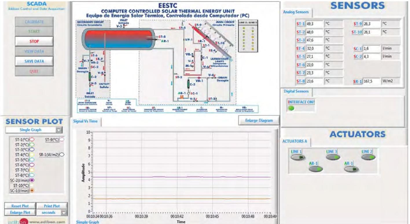
Time versus radiation emitted by the lamps on the solar panel.
